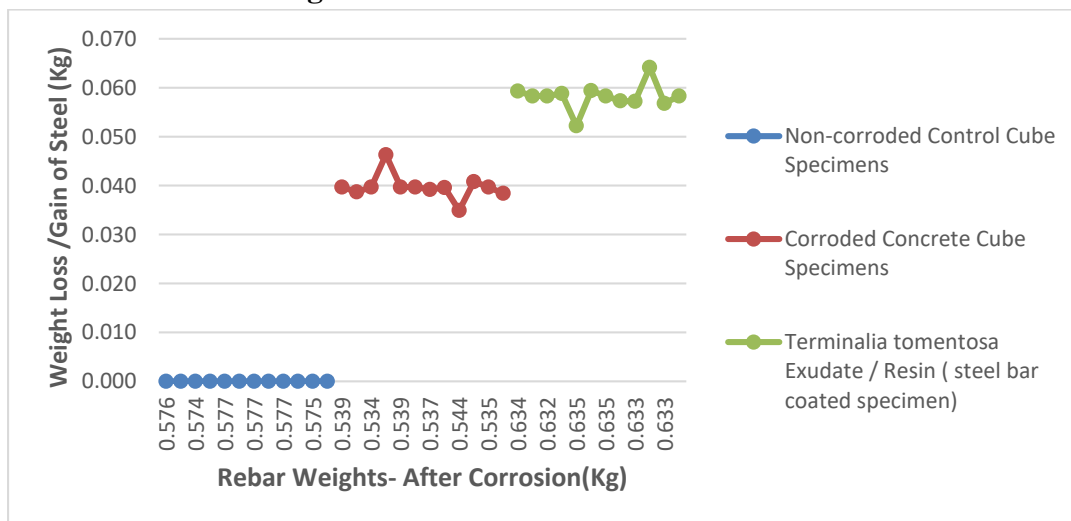
Figure 6. Rebar Weights- after Corrosion versus Weight Loss /Gain of Steel
